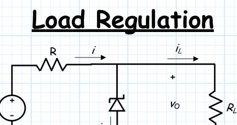
For voltage regulators, we typically define a load  $R_L$  in terms of its current  $i_L$ , where:
